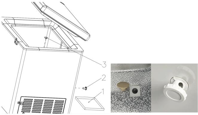
After using the product for a period of time, there may be condensed water formed at the bottom of the chamber, please drain away the condensed water in time to avoid damaging the storage items such as vaccines.
