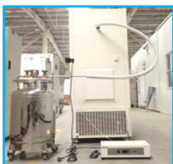
LN 2 /CO 2 backup system
