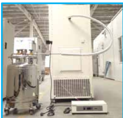
LN 2 /CO 2 backup system
