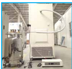
LN 2 /CO 2 backup system
